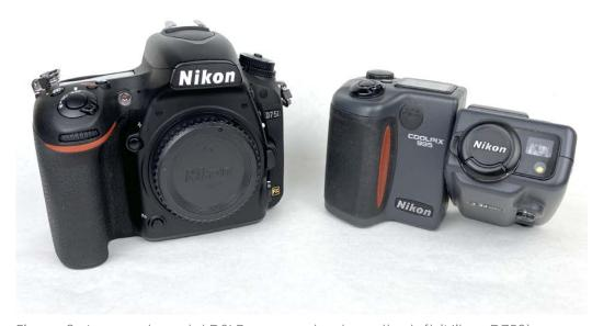
Figure 2. A current model DSLR camera body on the left (Nikon D750) and a vintage point and shoot camera (Nikon 995) from 2001. The 995, with its 3.34 megapixel sensor and excellent macro imaging firmware, was popular for numismatic photography a couple of decades ago.
