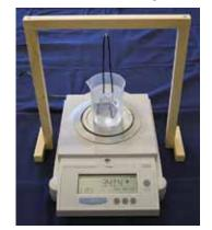
The SG apparatus above consists of a scale, a plastic container filled with water, a scaffold to suspend the coin, and a piece of plastic-coated wire bent to suspend the coin in the water without touching the sides or bottom of the beaker.
